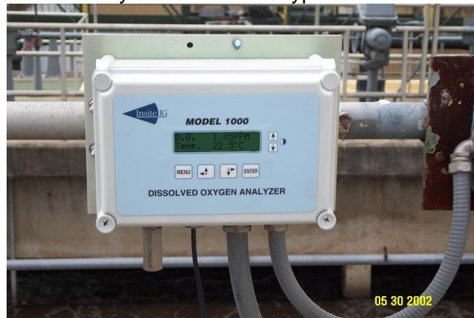
This in turn reduces hours of lost time for maintenance and eliminates the cost of replacement parts. Another very important feature is that fluorescent-based sensors do not consume oxygen and require no flow across them to work. They also perform very well in harsh environments that normally destroy other conventional sensors.
